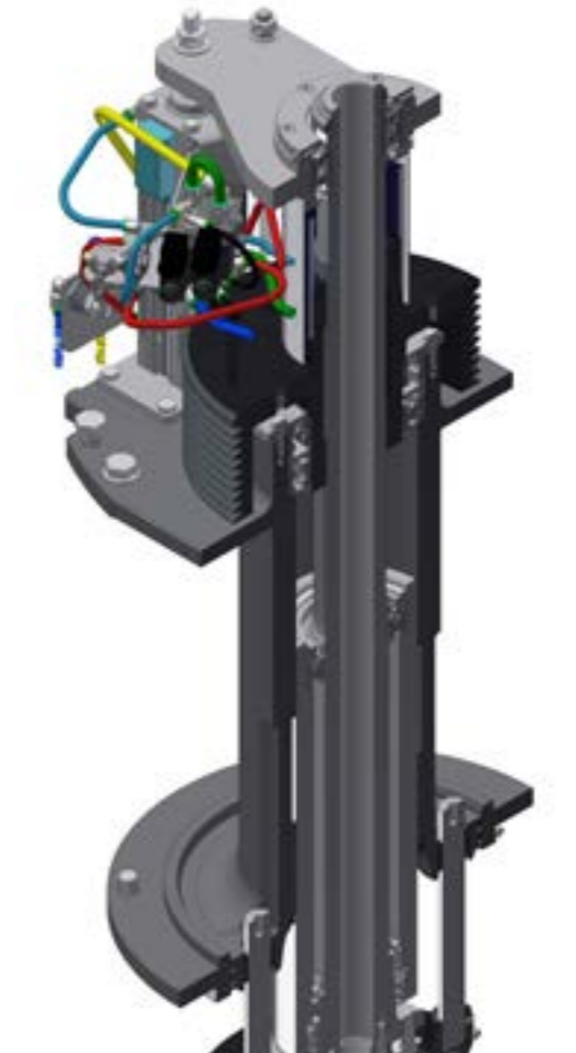
Oransal valf detayı – enkoderli silindir Detail of the proportional valve – cylinder with encoder
